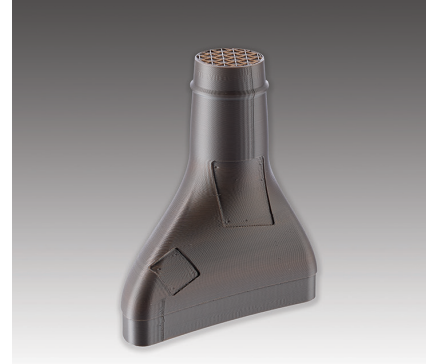
Figure 1: FDM sacrificial tooling begins with a 3D printed tool, which features a standard fill pattern designed to promote fluid flow during the tool removal process and provide adequate strength during elevated temperature, high pressure cure cycles.
