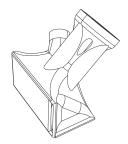
Parts: EOA Robotic Sander Model: ABS Print Time: 66h 15m This robotic sander is an end of arm tool that can be attached to a Universal Robots UR10e arm for automated hand sanding. The part benefits from the use of Stratasys® SR-30 dissolvable support, which allows for the design of an internal cavity in which sawdust can be channeled from the surface to a shop vac hose fitted to the exhaust vent.
